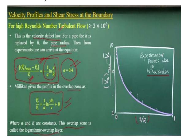
Now if you look it that, if you put it high turbulence flow and the velocity the reasons is very this is called velocity deflect law and h is replaced by the R the pipe radius then you can have this experimentally derived components and this alpha will represent a equal to the 0.4 and this is what the average velocity or time average velocity components and this is a special average velocity component how they are fluctuating with shear velocity.
