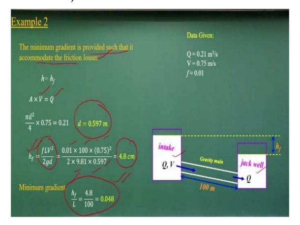
Another problems which is GATE 2014 questions also. A straight 100 meter long raw water, okay this only waters gravity main is carry the water from intake to a jack well okay of a water treatment plant okay. So basically there is a intake, to take the water from the rivers or ground waters and go to a well which is called the jack well where basic screening and all things turn it and then go for the water treatment plant.
