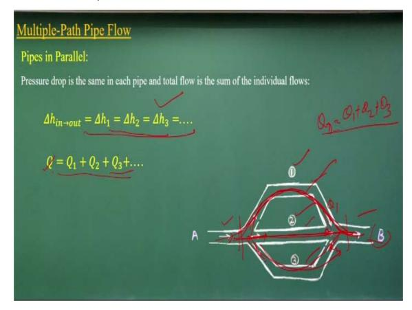
When you have a pipe in a parallels, you can understand it see if I have the pipe in the parallels, there are three pipes are connected here. This is the A is entry point, B is exit point. From the this point to this point the total energy losses passing through this path A or path B or path C that should be equal. So energy losses should be equal, whether it follows a path A, path B, or path C, all the energy losses should be equal.
