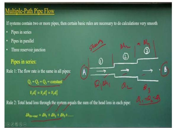
If you have definitely the discharge will be for a steady state conditions for steady flow conditions. So discharge at the Q<sub>1</sub>, Q<sub>2</sub>, Q<sub>3</sub> that should be equal because this is a steady state.
