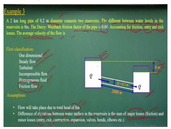
Let us start this third examples which is gives that 2 kilometer long pipe with a diameter of 0.2 meter diameter connects two reservoirs as given in the figures. The difference between the water levels in the reservoir is 8 meters. That means the energy losses between two reservoir is 8 meters. Darcy-Weisbach friction factor is given to us which is 0.04.
