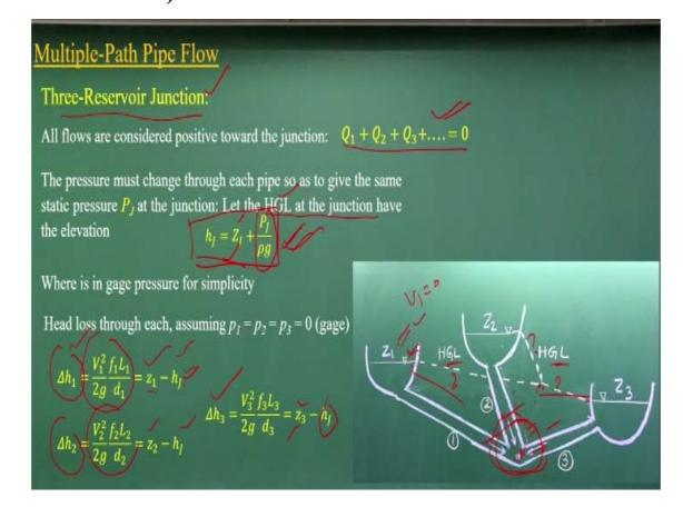
Now if you look it the three reservoir junction problems which many of the time it is given that you have a multiple reservoirs okay. You may have the multiple water tanks are there and connected to the pipe flow systems and you have a junctions where you have three are connected here. Out of these three flow one could be also outflow. We do not know that which direction it will be, outflow it.
