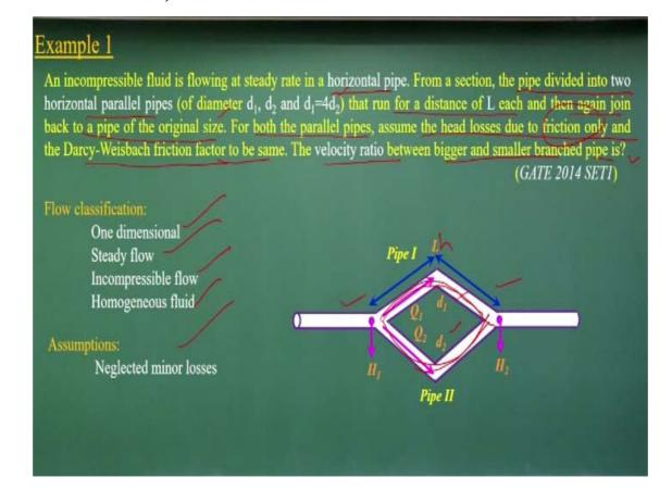
An incompressible fluid flowing through a steady rate in a horizontal pipe, okay. From a section, pipe is divided into two horizontal pipes as given the d 1 and d 2 okay and d 1 is four times of d 2 run for a distance l each other. Then again join back to pipe of the original size okay. We will just sketch the problem, okay? Many of the times please sketch the problems then you can understand it.
