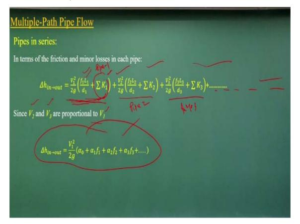
But when you have a pipe in a series please remember it that you always should consider whether there is a minor losses. There is major losses which is the frictional losses component for the pipe 1. Also there will be a minor losses because the change of the diameter of the pipe okay there will be expansion or the contraction exit loss, entry losses all the loss component you have to look it which way the flow is happening it and you can quantify what could be the minor losses.
